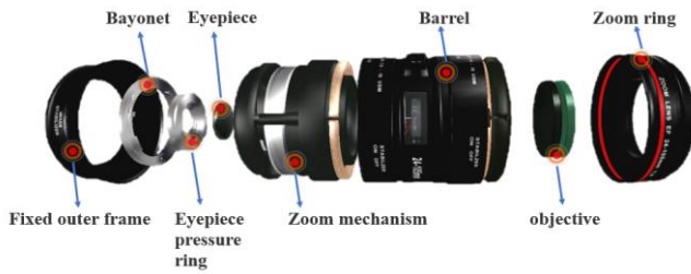
Figure 2: Parts list of the lens assembly
